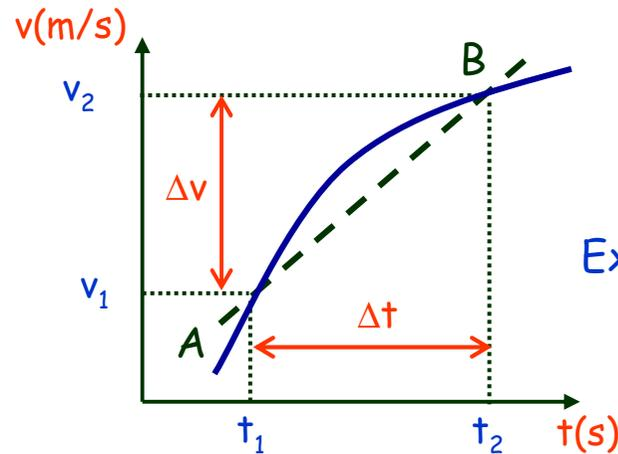
$$a_m = \frac{v_2 - v_1}{t_2 - t_1} = \frac{\Delta v}{\Delta t} \equiv \text{coeficiente angular da reta AB}$$
