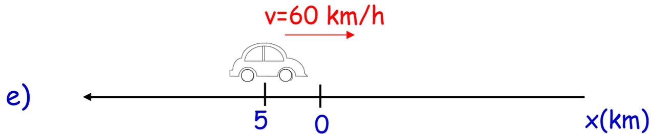
MRU  $\Rightarrow x(t) = x_0 + vt$  ;  $x_0 = 5 \text{ km}$  e  $v = -60 \text{ km/h} \Rightarrow x(t) = 5 - 60t$
