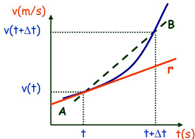
$$a_m = \frac{v(t + \Delta t) - v(t)}{\Delta t} = \frac{\Delta v}{\Delta t} \equiv \text{coeficiente angular da reta AB}$$
