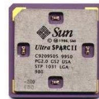
Sun UltraSPARC II Microprocessor
