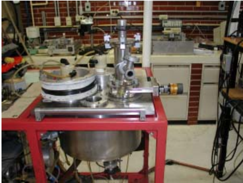
Figure 1. The chamber used to deposit the multilayers, with the coil concentric to magnetron.
