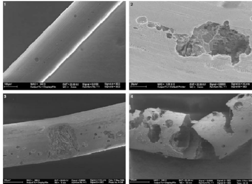
Fig. 5. Explanted nitinol struts from failed aortic stent grafts.<sup>4</sup> The arrow represents approximately a 100  $\mu$ m scale. The large surface pits seen in the top right and bottom left are likely responsible for the failures seen in the bottom right. The surface pits are likely expansions of the defects seen in Figs. 3 and 4. Figure from Ref. 4; reproduced with permission.
