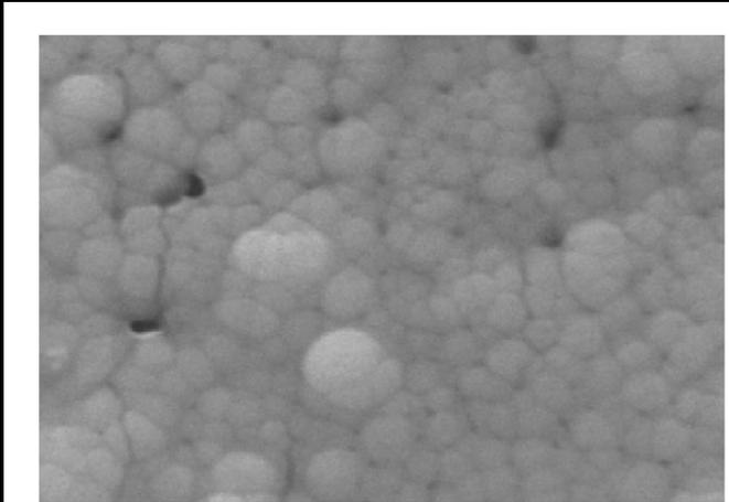
Fig. 7. The surface of a medical device coated with a nickel-phosphorous alloy deposited via electroless deposition. The white calibration bar represents 500 nm. Bioactive materials can be incorporated in between the grains. Courtesy of Nanomedical Technologies, Inc.
