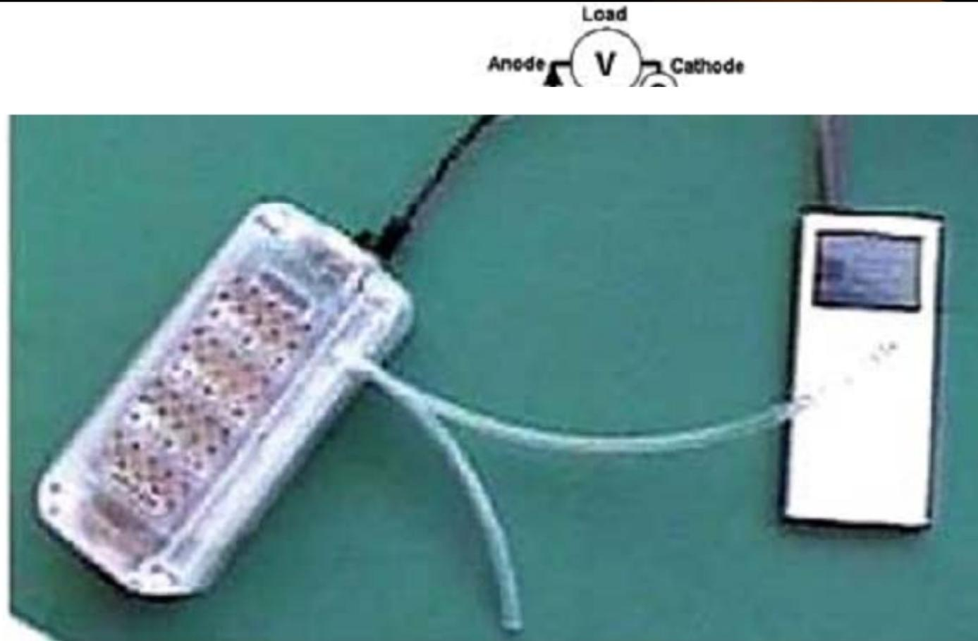
**FIG. 4.** Ethanol/air biofuel cell stack. This prototype, developed by Akermin, Inc. in 2006, powers an iPod. Photograph courtesy of Akermin, Inc.
