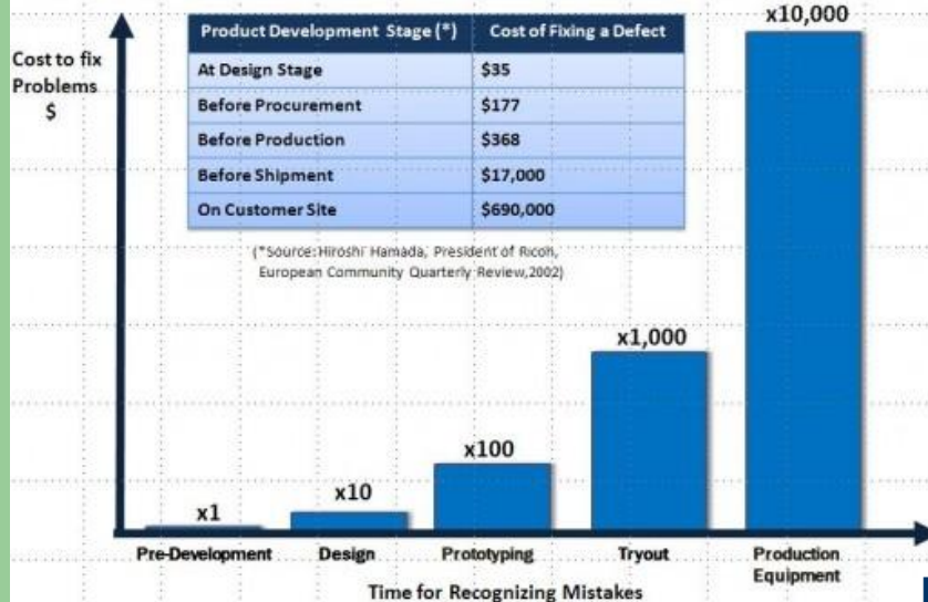
The Cost of Reliability - fixing mistakes in product design at different developmental stages (Ricoh)
