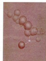
Figure 6 - Agglomeration of alpha particles tracks originated from the ^{10}\text{B}(n,\alpha)^7\text{Li} reaction in CR-39
